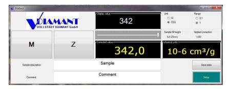
The radio buttons for unit and range must be set according to the physical settings on the MS2.
