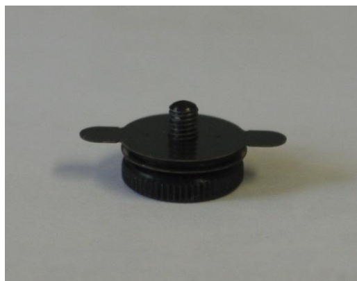
Picture 9: assembled pressure chamber; if mounted horizontally the 0.2 mm orifice is in function, if mounted vertically the orifice is 0.3 mm)
